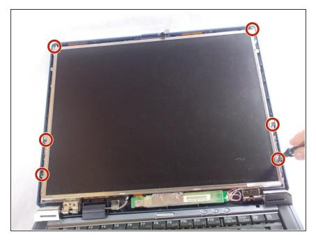
Remove the six screws along the outside of the screen using the PH 0 screwdriver bit.
