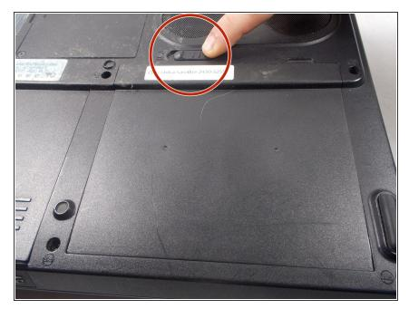
Locate the battery locking mechanism on the back side of the laptop. It is labeled with a lock and unlock symbol to indicate its function. The mechanism also has a serrated texture to increase grip.
