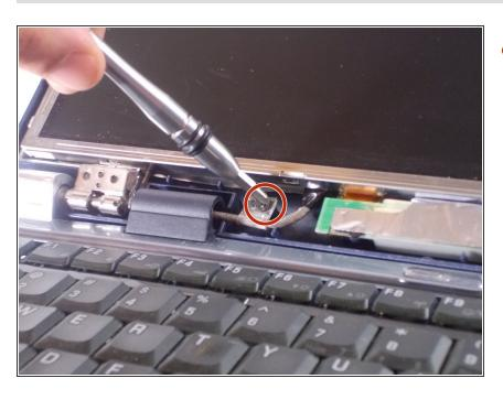
Next remove the screw holding down the white wire using the PH 0 screwdriver bit.
