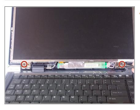
Remove the two screws holding the screen to the frame using the PH 0 screwdriver bit.
