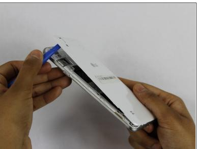
Insert a fingernail, or plastic opening tool, into the cutout on the back cover and pry outward to remove.
