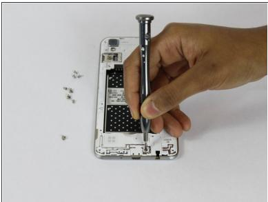
Remove the twelve 2mm JIS #00 screws from the mid-frame.
