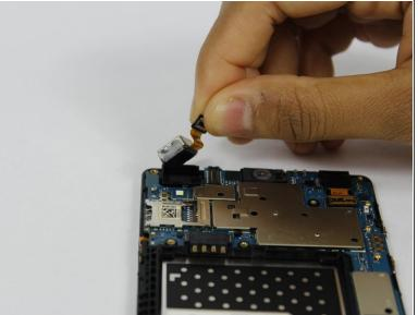
Use a plastic opening tool to disconnect the rear camera and pull from the phone.
