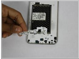
• Using a plastic opening tool, remove the antenna extender from the mid-frame.
