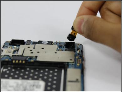
Use a plastic opening tool to disconnect the front camera from the motherboard and pull out to remove. To reassemble your device, follow these instructions in reverse order.
