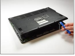
• Use a plastic spudger to pry up the bottom cover and remove it.
