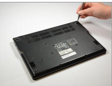
Use a Phillips head screw driver to remove the 13 screws in these locations.
