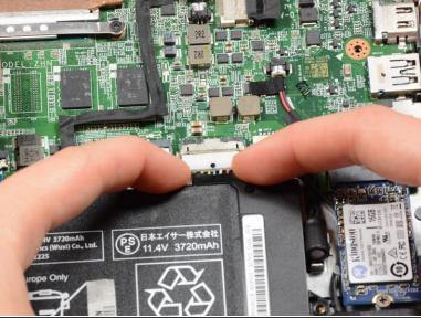
Use two fingers to unplug the battery-to-motherboard connection.
