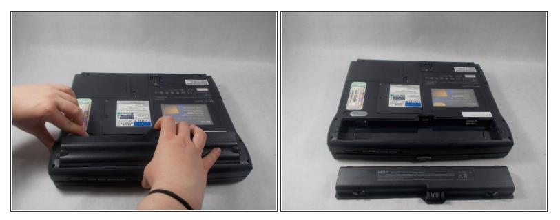
• While continuing to hold the finger latch, slowly lift up on the tab to remove the battery from the device.
