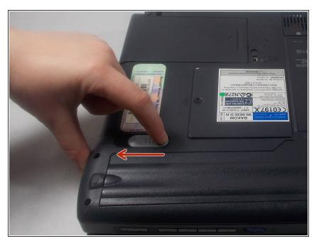
• Slide the finger latch to the left to release the clip holding the battery into the laptop.
