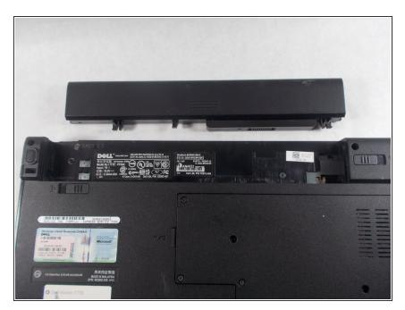
Remove the battery from the slot.
