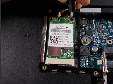
• Remove the two 3mm Philips #1 screws from the top of the Wi-Fi card.
