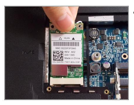
Gently pull Wi-Fi card out of its position at its angle.
