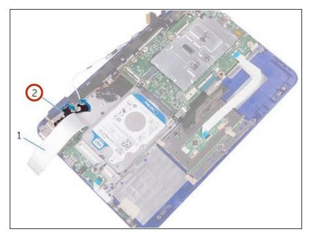
Peel the tapes off the display hinges.
