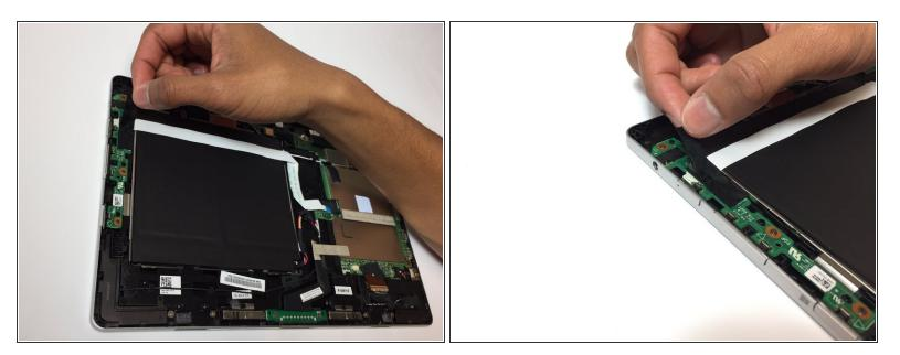
Remove the piece of black, thin tape that is attached to the circuit board closest to the power button.
