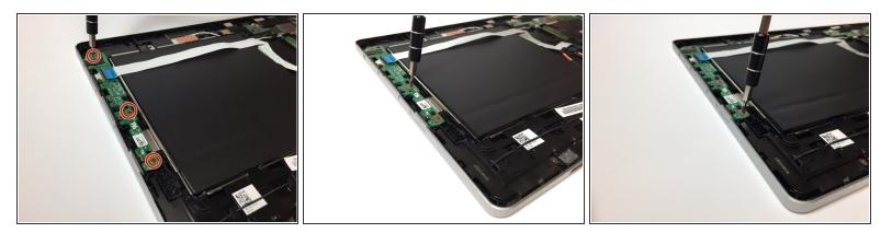
• Use the Phillips #000 screwdriver to remove the three 3 mm screws on the circuit board.
