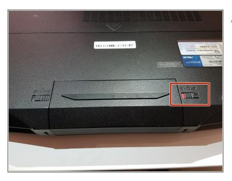
Unlock the battery by pushing the switch to the right.
