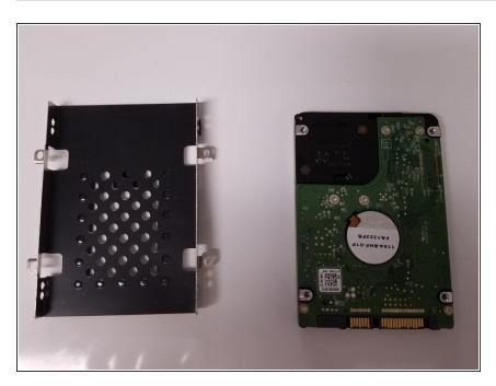
Slide the hard drive out of the casing.
