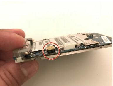
• The charging port is soldered to the motherboard, use this guide to do the replacement.
