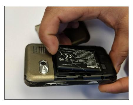
Remove the battery by levering the battery out, using the cut just below the camera.
