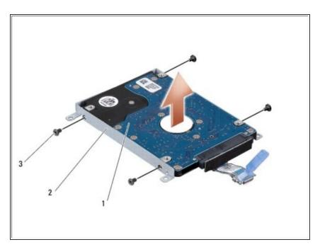
• Remove the four screws that secure the hard drive bracket to the hard drive and remove the bracket.
