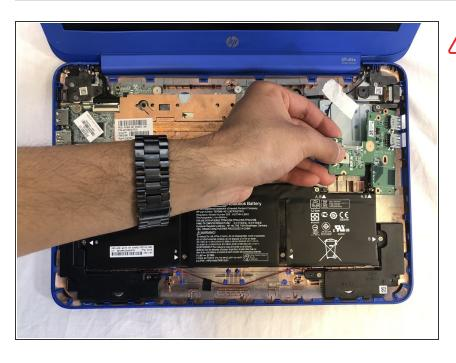
Remove the chip containing the two USB Ports.
