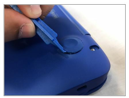
Remove the five rubber feet from the bottom of the laptop with a plastic opening tool.
