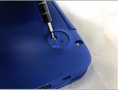
• Remove the thirteen 5mm Phillips #0 screws from the bottom case.
