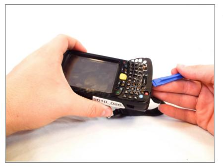
Use a plastic opening tool to remove the keyboard cover by prying up on its perimeter.
