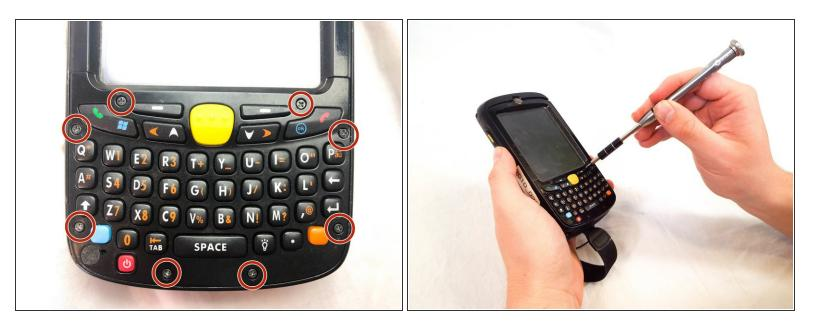
• Remove the eight 4mm Phillips #00 screws from the keyboard cover.
