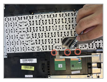
Remove the three 3mm Phillips #0 screws from the touchpad.
