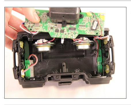
Gently pull the battery from the housing of the device while disconnecting the red, white and black wires coming from the battery.
