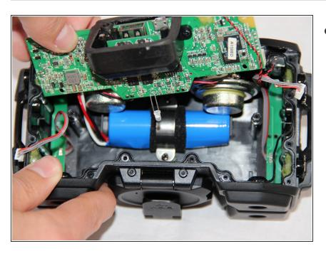
Once disconnected, carefully remove the motherboard by pulling upwards.
