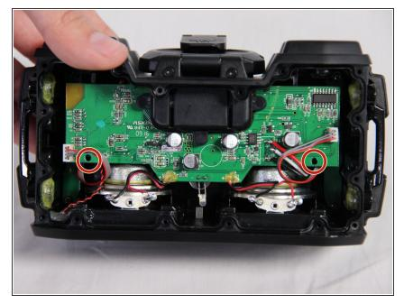
To remove the motherboard, proceed to unscrew the 3 Phillips #00 bit type, 13mm long screws located on both sides of the motherboard.
