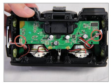
Disconnect the two 4-pin auxiliary button register cables connected on both sides of the motherboard.
