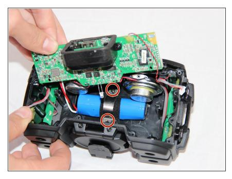
To remove the battery, unscrew the 2 Phillips #00 bit type, 9 mm long screws on both sides of the battery.
