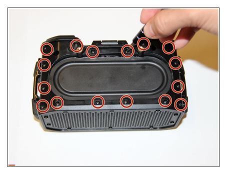
To remove the inner plastic casing, use a Phillips #00 head bit to remove the 16 small 9mm screws surrounding the top side of the device.
