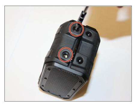
To remove the outer casing, use a 3mm Hex bit to remove the 4 large 12mm Hex screws on both sides of the device.
