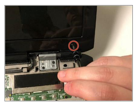
Remove 2 M2x3mm screws that are located at the bottom of the plastic bezel with a PH0 screwdriver.
