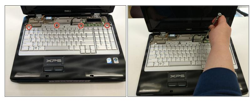
Remove the four screws from the top of the keyboard bracket.
