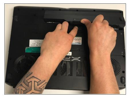
Slide the button next to the battery and lift up on the lip of the battery edge.
