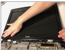
Use iFixit plastic tool and a cutout of cardboard to pry out the plastic bezel around the edges of the LCD screen
