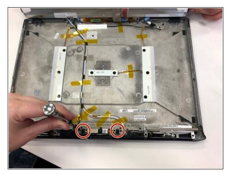
Remove the four screws (M2x3mm) surrounding the webcam
