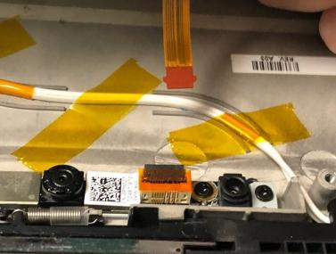
• Disconnect the display connector behind the top of the screen.
