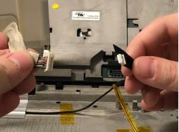
Disconnect the display connectors by removing them from the grooves and unplugging them.
