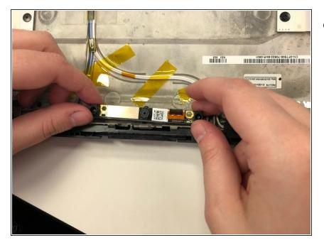
Lift up on the webcam bar to pull it out.
