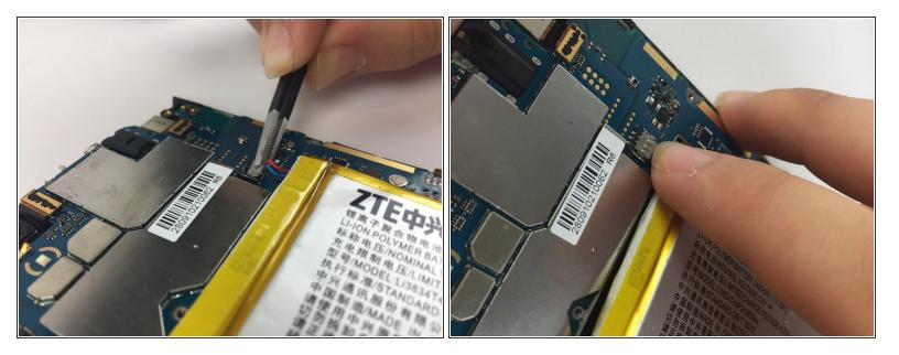
Disconnect the battery from the motherboard.
