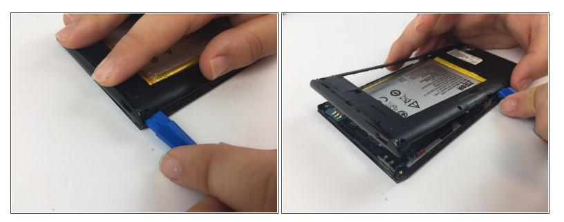
Remove the mid frame with the plastic opening tool.
