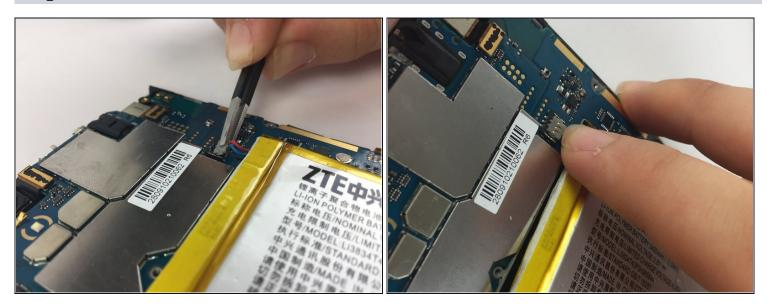
• Disconnect the battery from the motherboard.
