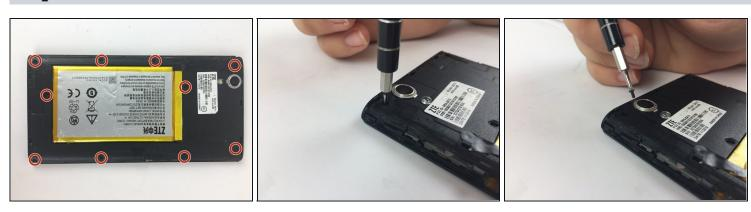
• Remove the ten 1.2mm screws with a Phillips #000 screwdriver.
