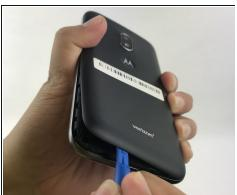
Open case with a plastic opening tool that has the same size as the divot located at the bottom left of the phone. If you don't have an opening tool, use your finger nails.
