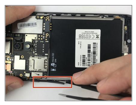
Remove the volume button by pushing the round tips out using the tweezers (or a pen if you don't have tweezers).
