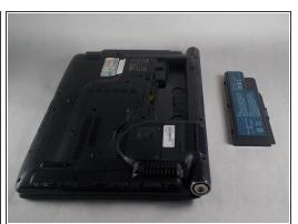
Pull the battery up and out. Use a plastic opening tool if necessary.
