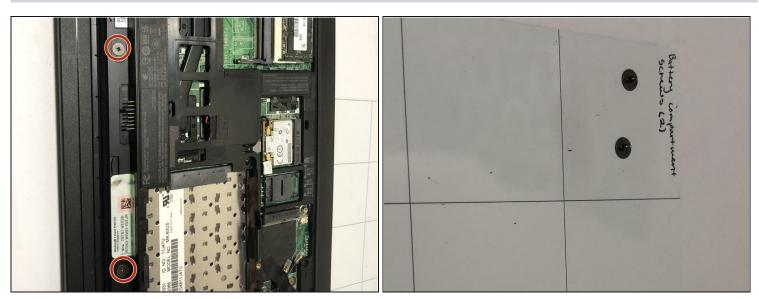
• Remove the two retaining screws where the battery is located. Set the two screws aside on the <u>magnetic mat</u> and label one square "battery compartment screws (2)" like so.
