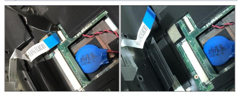
• using the pryer, pull the little black tab above the blue ribbon up, now you should be able to pull the wires straight out and fully remove your keyboard.
