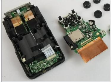
Gently lift the motherboard from the base of the device and set aside.
