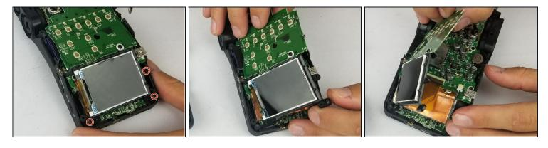
Unscrew three (PH #1), 7mm screws from the display backing and gently flip over.
