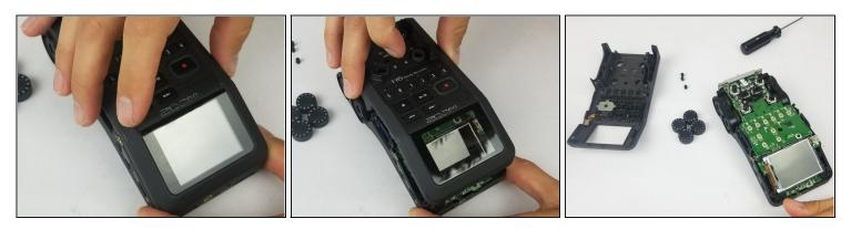
• With the bottom of the device on a table, lift the top of the device and gently place it aside.
