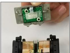
• Lift the mic connector out of the base of the device.
