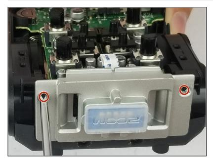
Turn device 180 degrees to unscrew two (PH #1), 8mm screws from the mic connector.
