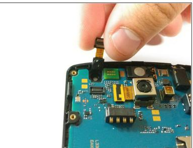
Unclip the front camera connector from the motherboard and lift it from the frame.
