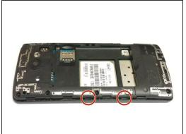
Use an opening tool on the marked locations to lift the edges up. There should be a small click when lifting these edges up.
