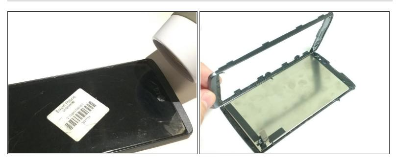
Using a hot air gun or hair dryer, heat the screen assembly, and pry it from the frame using your fingers (or an iFixit prying tool).
