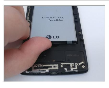
Place your thumb along the bottom of the battery and pry upwards to remove.
