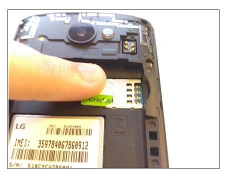
Press down on the SIM eject tab with a fingernail (or iFixit opening tool), and slide the SIM card out.
