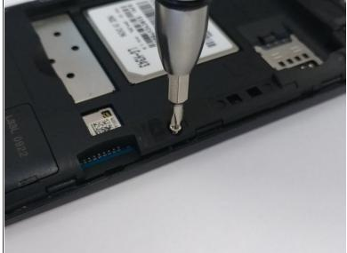
Remove the eight Phillips #0 screws from the internal support frame.
