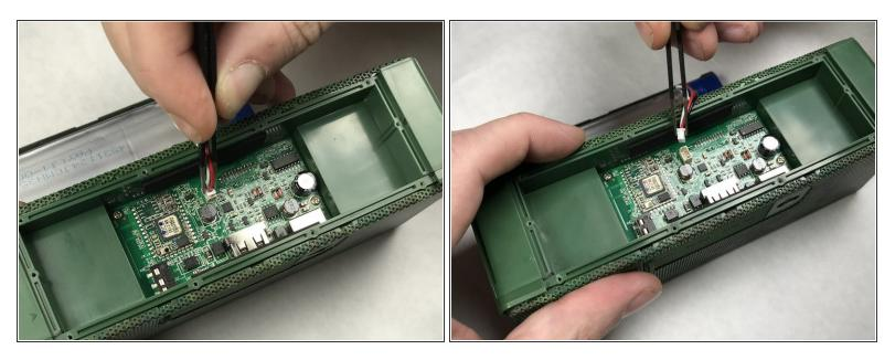
Using tweezers, carefully detach the battery wire from the circuit board and lift out the panel with the attached battery.
