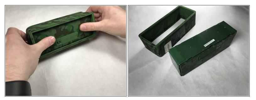
• Turn the device around and gently push the speaker through until it separates from the sleeve.
