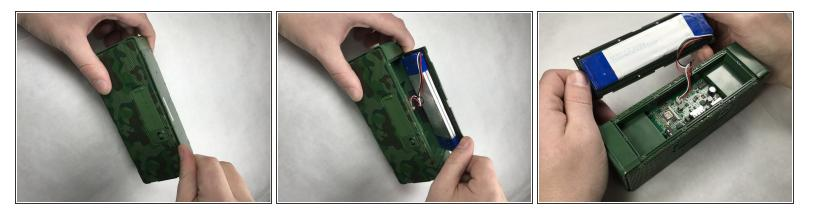
Using your hands, pry the panel off of the top of the device to reveal the device circuit board and the battery attached to the inner side of the panel.
