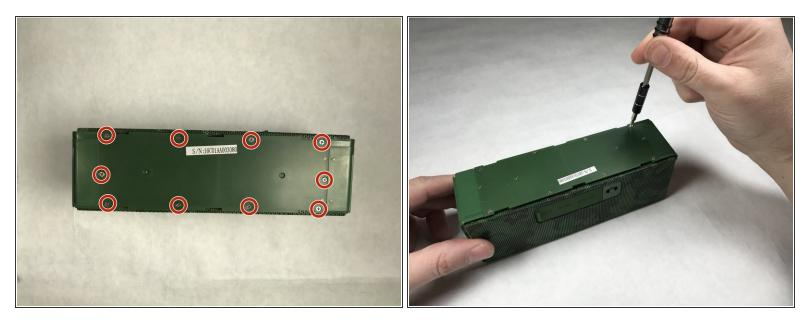
Using a Phillips #0 screwdriver, remove the the ten 5.1mm screws that hold down the battery panel on the bottom of the speaker unit.
