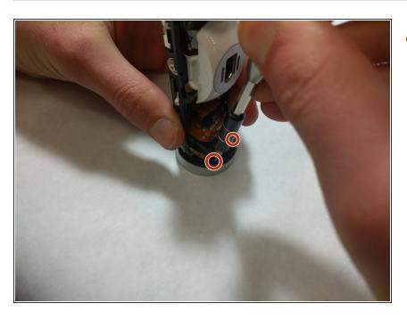
Unscrew 2 (4.41 mm) screws seen in the picture that surround the attachment of the lens to the main body.
