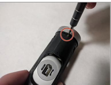
Unscrew the 3 (3.55 mm) screws surrounding the black casing near the camera-lens.
