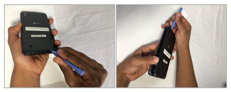
Insert a plastic opening tool above the AUX jack and slide it around the perimeter to pop the back cover off.
