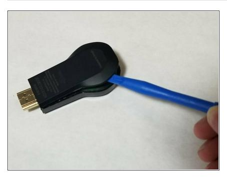
Continue prying the top of the case from the bottom toward the HDMI port until the top casing is completely removed.
