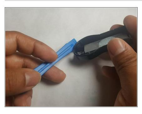
Press the plastic button from the outside of the port, pushing it inward if it is stuck. To reassemble your device, follow these instructions in reverse order.
