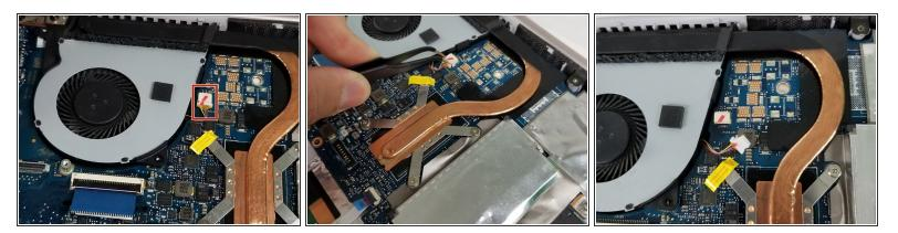
• Using tweezers, disconnect the cable connector from the motherboard fan.
