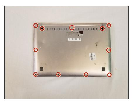
Remove the eleven 4 mm Phillips #00 screws from the back panel.
