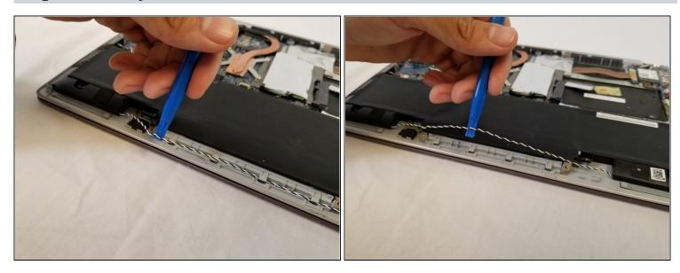
• Pull the speaker cable out of its four retaining clips with either your fingers, or a plastic opening tool.
