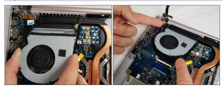
• Lift the fan up and off of the white pegs that secure it into place.
