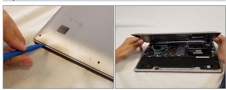
• Using a plastic opening tool pry the back panel off of the laptop.
