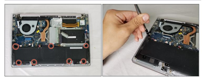
• Remove all seven 2 mm Phillips #00 screws from the battery.
