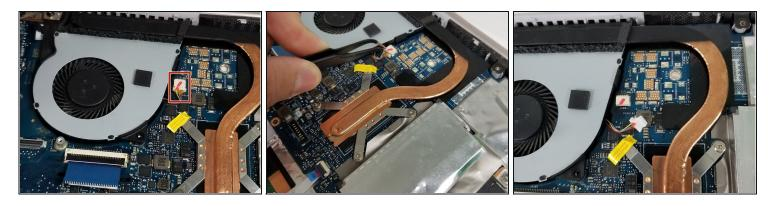
• Using <u>tweezers</u>, disconnect the cable connector from the motherboard fan.
