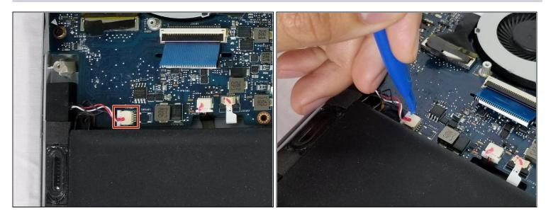
• Pull the speaker connector toward the edge of the laptop to disconnect it from its socket.
