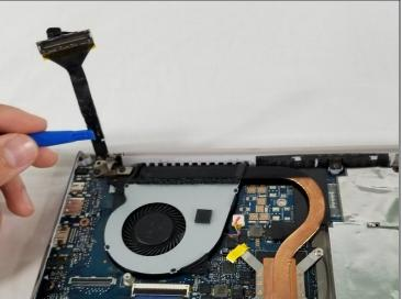
• Disconnect the display cable from the motherboard with a plastic opening tool.
