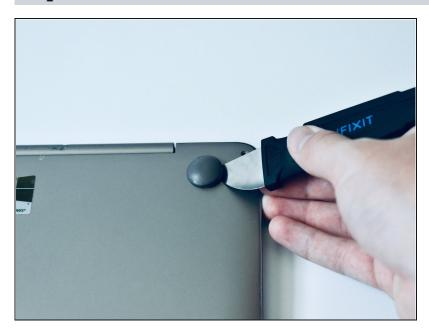
Remove the two round rubber feet at the hinge-edge of the laptop.
