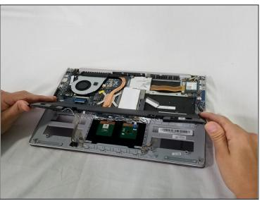
Lift the battery and speakers up and pull out to remove.
