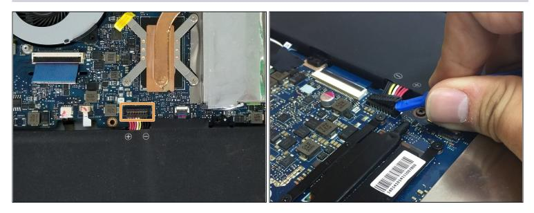
• Lift the battery connector straight up off its socket to disconnect it from the motherboard.
