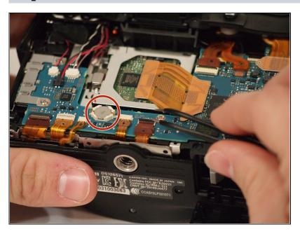
Remove the button cell battery from the motherboard using a pair of tweezers.
