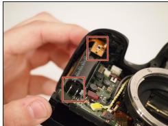
• Using the plastic opening tool, pry the front of the casing off of the camera.
