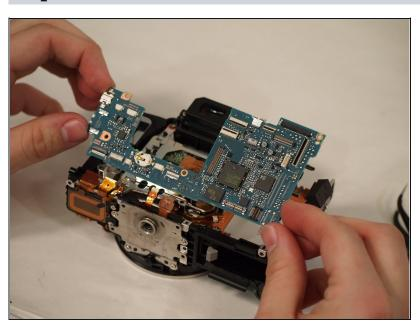
• Remove the motherboard from the device.
