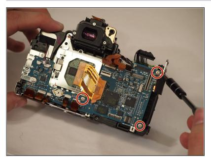
Remove the two screws on the right side of the motherboard as well as the screw in the center.
