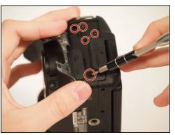
• Using a metal spudger, pry the rubber grip off of the casing on the left side of the camera.
