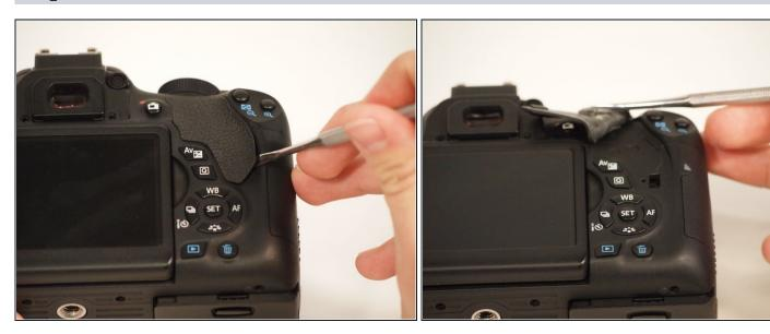
• Using the metal spudger, pry the rubber grip located just below the turndial.
