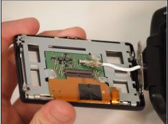
• There are several components inside the casing. A board, a power cable, the screen and a ribbon cable. First, using <u>tweezers</u> lift the metallic clamp connecting the ribbon to the board.
