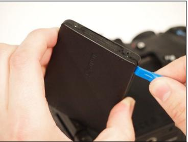
• Following the removal of the 6 screws, Locate the joint of the casing. Place a flat lever inside this crevice and apply pressure. The case should simply pop open into the 2 casing pieces and the screen mechanism. Warning. No Dot try to remove bottom casing until next step.
