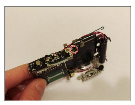
Remove the 3mm black screw from top of the camera light.
