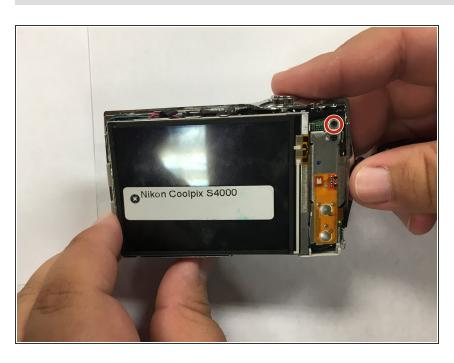
Remove the single 3mm Phillips #000 screw from the back of the camera.
