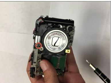
Remove the two 3mm Phillips #000 screws.
