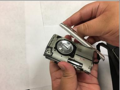
• Use your fingers, or a spudger, to lift up one end of the casing and then pry the two pieces apart.
