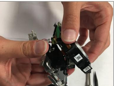
Use the flat end of a spudger to pry the lens locking tabs open while pulling the lens away from the camera body.
