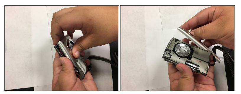
• Use your fingers, or a spudger, to lift up one end of the casing and then pry the two pieces apart.
