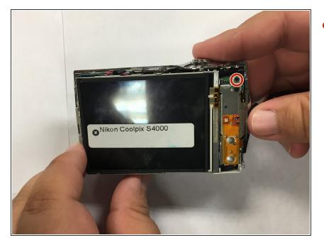
Remove the single 3mm Phillips #000 screw from the back of the camera.
