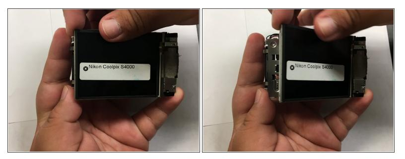
• Grabbing the top left corner of the screen, pull it up until the screen comes completely off.
