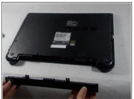
Once the screws are removed, slide the battery pack out of the computer.
