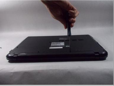
Remove the two 6.5 mm Phillips head screws indicated using a Phillips #00 screw driver.
