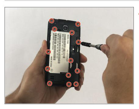
Remove the thirteen 3mm Phillips #00 screws from the back panel.
