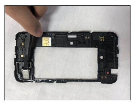
Use the flat end of a spudger to lift the speaker out of the frame and remove.
