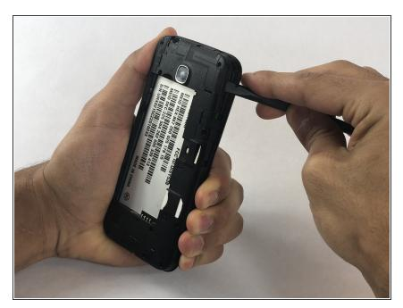
• Use the flat end of a spudger to pry off the back panel.
