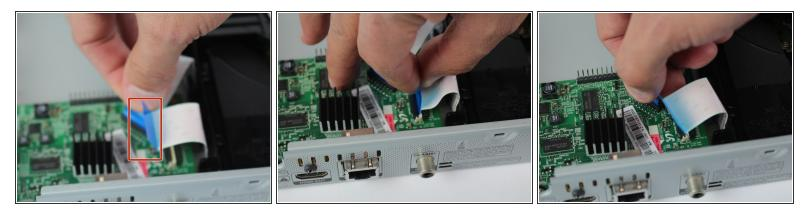
• Grip the blue tab and pull upwards to remove the ribbon cable from the motherboard.
