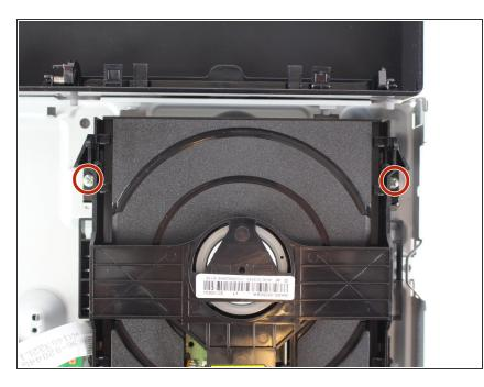
Remove the two 7mm screws with a Phillips #1 screwdriver.
