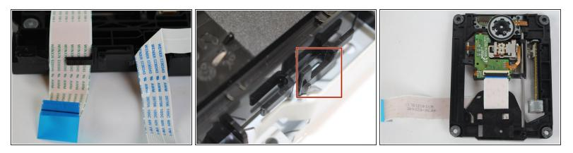
Pinch both tabs on the side of the disc tray, push towards the front, and lift the disc tray out to remove.
