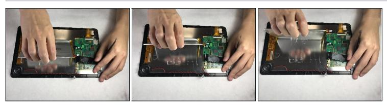
• Carefully peel off the battery.
