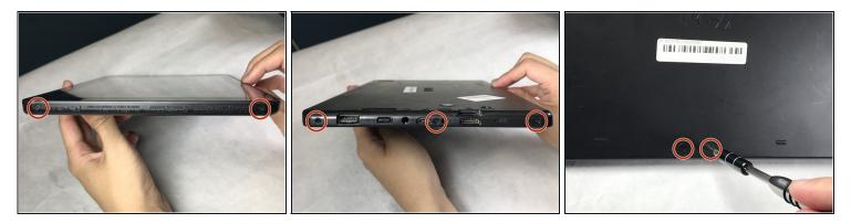
• Remove nine 4.8mm screws around the case with a JIS #00 screwdriver.
