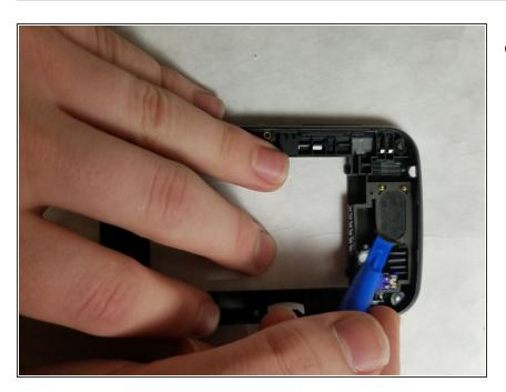
Insert plastic opening tool under the plastic flap and lift the speaker out.
