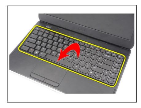
• Flip the keyboard over and lay it on the palm rest.
