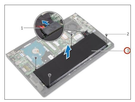
Lift the battery, along with its cable, off the palm-rest assembly.
