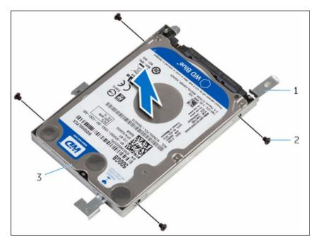
Align the screw holes on the hard drive with the screw holes on the hard-drive bracket.
