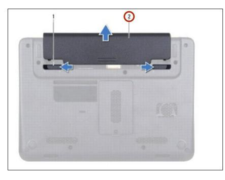
• Slide the **NEW** battery into the battery bay, until it clicks into place.
