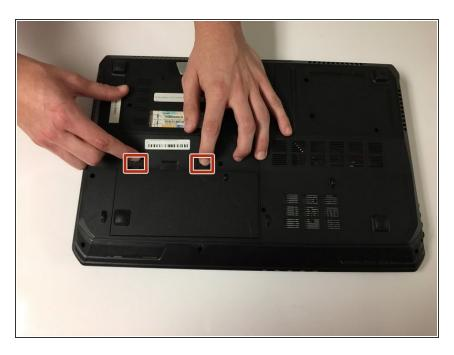
Pull the latches away from the battery compartment. The lid of the compartment should pop out of place.
