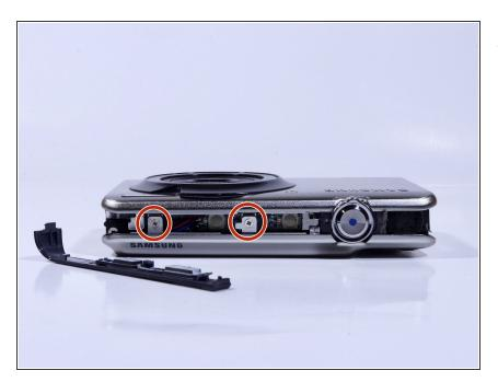
Remove screws beneath the top panel indicated by red circles with a #00 Phillips driver.
