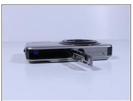
Unlock the battery compartment by sliding the switch to the open position.
