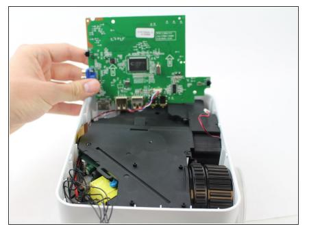
Raise motherboard by lifting sideways and then up to avoid the ports.
