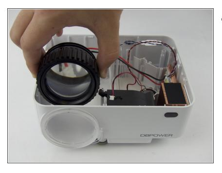
Remove the focus-adjustment ring from the lens housing.
