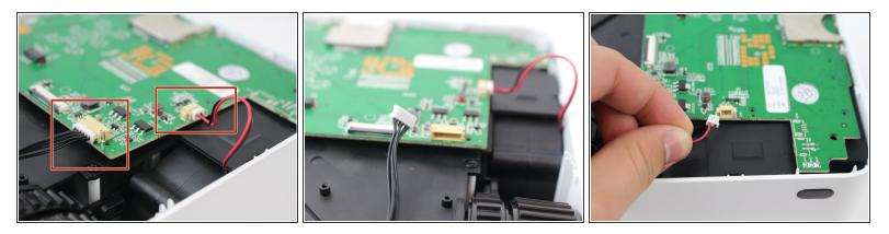
• Remove the two cables connected to the motherboard: black power cable and the red/black fan cable.
