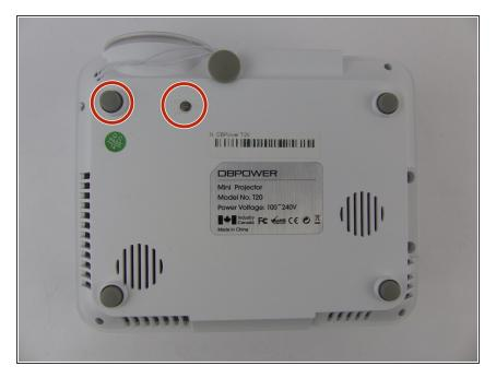
Remove the rubber foot and warranty sticker found underneath the device.
