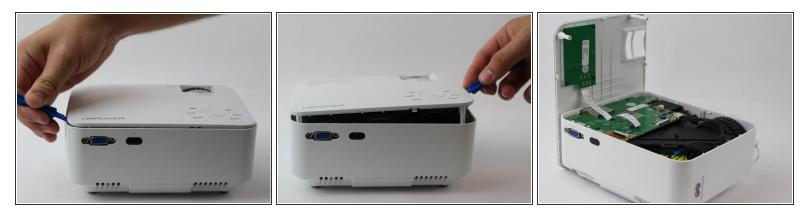
• Flip the device over and pry the top off with a plastic opening tool.
