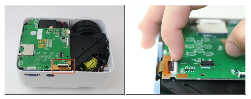
• Lift the black latch on the ZIF connector and remove the ribbon cable that attaches the digitizer to the motherboard.
