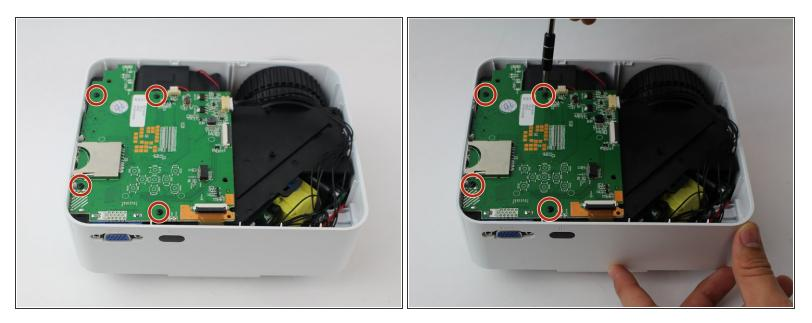
• Remove four (6 mm) screws connecting the motherboard using a J0 screwdriver.
