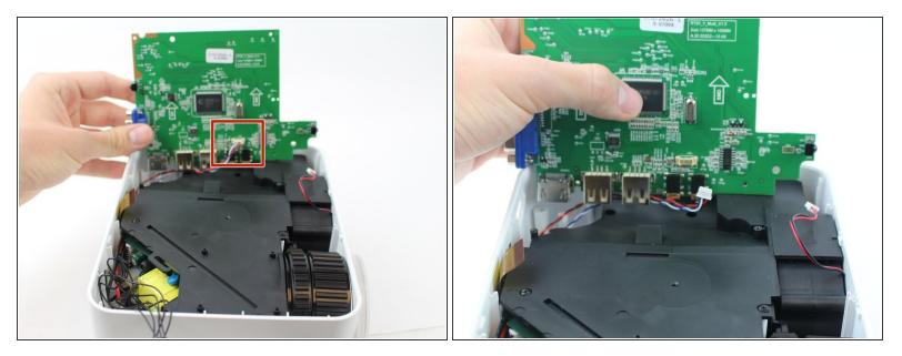
• Remove wires attaching the piezoelectric speakers to the motherboard.
