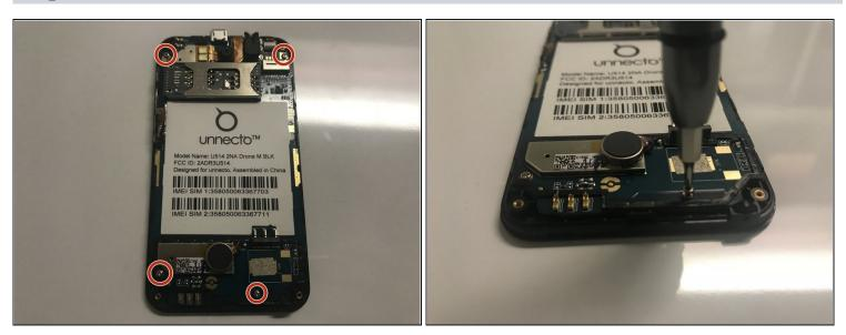
• Use a Phillips #000 screwdriver to remove the four screws that secure the motherboard.
