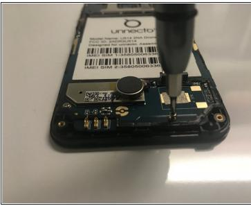
• Use a Phillips #000 screwdriver to remove the four screws that secure the motherboard.
