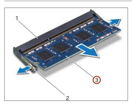
Slide the memory module firmly into the connector at a 45-degree angle and press the memory module down until it clicks into place. If you do not hear the click, remove the memory module and reinstall it. To reassemble your device, follow these instructions in reverse order.
